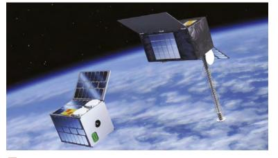
LEO-PNT is the first project in which GMV takes on leadership of a complete space mission, including the development and manufacture of the satellites. The goal of this demonstration mission is to develop technology for the provision of more accurate positioning, navigation, and timing services through the launch of a low-orbit satellite constellation.
