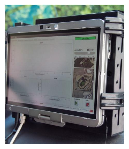
CORPAC S.A., Peru's air navigation services provider, has recently procured calibration equipment with *Emil*, GMV's inhouse system for ground inspection of ILS and VOR radio aids.
