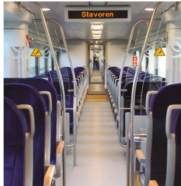
Current and next station information is shown on on-board displays and/or on-board monitors. The related audio speech is simultaneously broadcasted through the PA system of the train.
