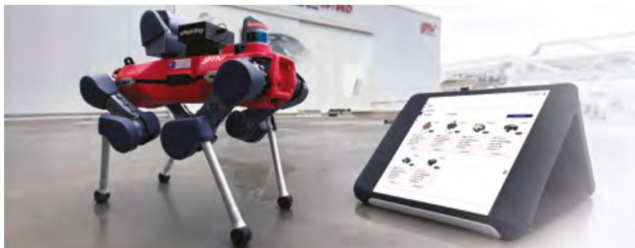
Led by Elewit and Red Eléctrica (both part of the Redeia group), ASUMO embodies the vision of a smarter industry by integrating *uPathWay* into a quadruped robot capable of autonomous missions: from reading analog indicators and conducting thermographic reports to detecting oil leaks and tracking discharges.
